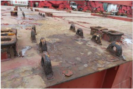
Pictures of other deficiency: FORWARD NATURE VENTIALTOR FOR NO.2 CARGO HOLD FOUND SEIZED, AND AFTER SIDE NATURE VENTILAOR FOR IT FOUND INOPERABLE.
